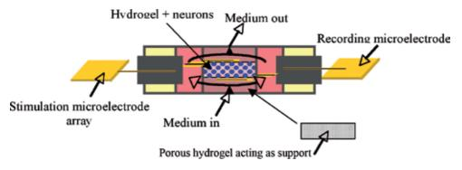
Figure 10. Cross section of the perfusion bioreactor with hydrogels containing neurons interfaced with two microelectrode arrays.
