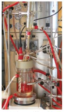
Figure 7. 3D bioreactor with fully controlled conditions.
