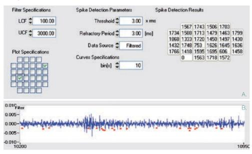
Figure 6. Screening of spikes, numbers in the boxes, detected in one minute by each one of the 32 microelectrodes of the array (a), shows high activity. Part of the recorded signal from one of the microelectrodes (b). Spikes are detected after removing the noise of the signals and are indicated with red dots in (b).
